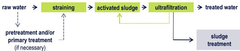
Ultrafor™ incorporates biological treatment by activated sludge with clarification by immersed membrane ultrafiltration. Water to be treated enters a reactor where it is put in contact with a purifying bacterial mass before passing through the membranes.
