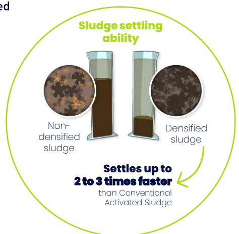
This process progressively increases the quantity of the most efficient organisms in the biological reactor at the expense of the less efficient forms that are extracted. This densified biomass has a superior settling ability compared to Conventional Activated Sludge, maintaining a stable and low Sludge Volume Index (SVI) throughout the year, regardless of adverse weather conditions. It limits also the escape of suspended solids, thus improving the quality of the treated water.
